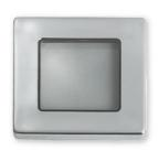
Techno-polymer body.. Silicone gasket for the glass.. Satiny, tempered White glass.. Techno-polymer flange... AISI 316 L ring.. Aluminium heatsink. Inside screws in stainless steel. . Directional reflector aluminium metallised. Supplied with LED power module 3x1W and integrated regulator. Supplied upon request with LEDs modulus white and red, white and blue. White colour 3200 °K degree. Suitable for mounting on normally flammable surfaces. Can be supplied upon request with white Leds
