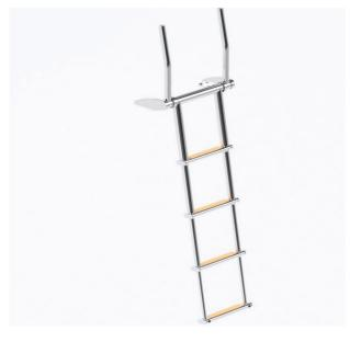
Over platform telescopic boat ladder made of mirror-polished AISI 316L stainless steel for boats and ribs with 4 steps and retractable and self-erecting handles. The handles move up and down automatically only by rotating the ladder and simplify boarding from the water and ladder recovery when onboard. Steps in oval stainless steel have a water-draining hole, welded stainless steel lateral sealing caps and are available with non-skid pads or wood splint.
