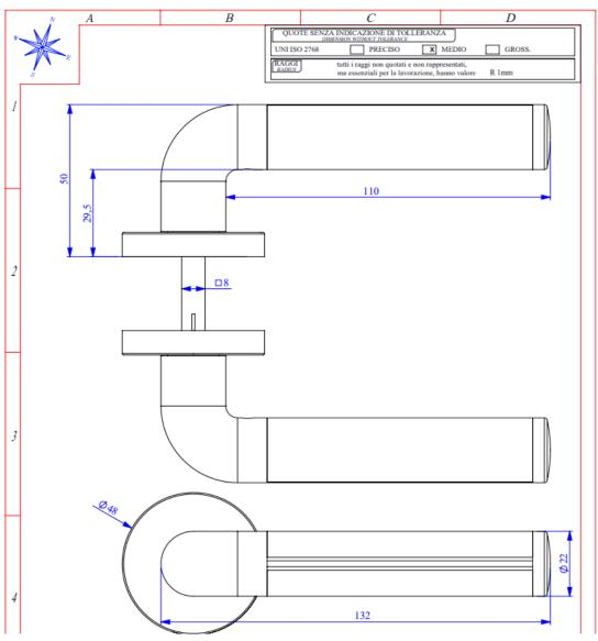
Base Diameter (mm) 48.00 Spindle (mm) 8.00 Spindle Length (mm) 80.00 Protrusion (mm) 52.00 Handle Length (mm) 130.00 Manufacturer Foresti & Suardi Weight (kg) 0.60
